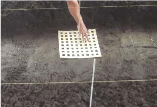
Figure 2: Bamboo grid reinforcement models
